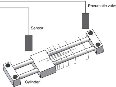
All data can be converted to electronic format and, by combining with an OMRON PLC (CS/CJ Series), checked directly from Ethernet or the Internet to allow remote maintenance.
