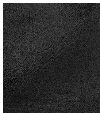
Neutrarust 661® Technolo- gy 2 coats - 750 hours salt fog cold rolled steel
