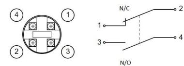
The switch is not polarity sensitive
