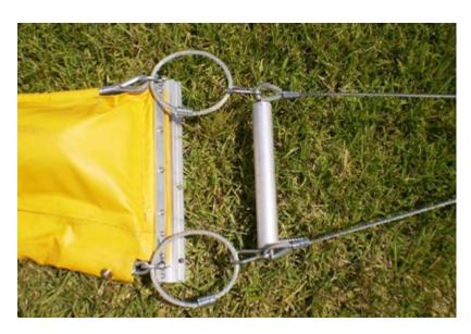
An option, extra cable anchor loops can be fitted at regular intervals along the boom, top and bottom, to provide additional anchor points. A special tow bridle with spreader bar prevents the boom skirt from collapsing. Attached to the cable anchor loops with quick connect snap hooks.
