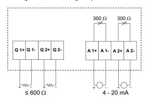
You can configure the following analog outputs on your meter through communication only:
