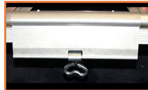
3. Place the WingSpan on the top rung of the ladder when the ladder is in extension position only. Make sure the WingSpan is centered securely on the top
