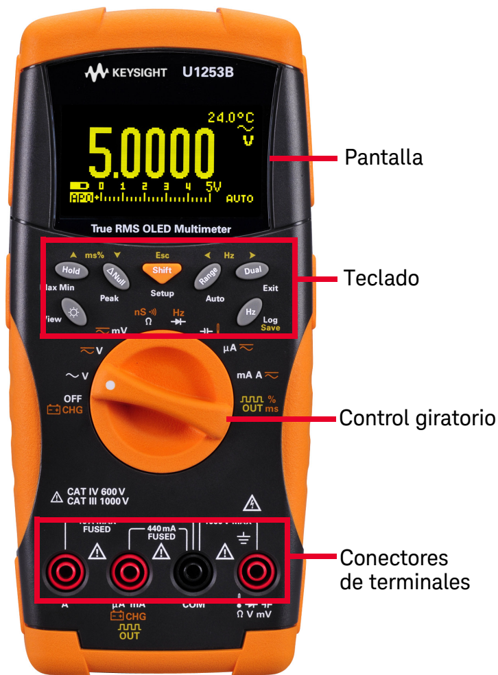
Figura 1-4 Panel frontal del U1253B
