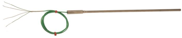
Duplex Type 'K' Thermocouple with two independent measuring junctions inside tip of probe. This allows one probe to be connected to two measurement or control devices; alternatively, one sensor may be used as a primary and the other as a backup, eliminating the need to remove and replace the probe if one of the sensors should fail.
