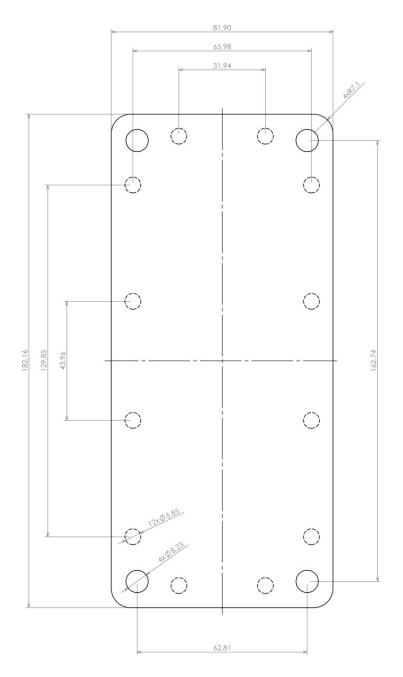
Dashed line shows outline of the mounting boss under PCB board Recommended mounting holes diameter ø3,5mm All dimensions are given within +/-0,5mm tolerance
