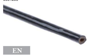
Made of silicone rubber coated fibreglass braid with a unique construction that allows the sleeve to expand up to 1.6 times its original size. This allows it to expand over awkward shapes and 'conform' itself to the profile of the part it is covering. This sleeving is often used as an alternative to heat shrink as it requires no heat or mechanical tools for installation; it simply slips over whatever shape you need to cover for a perfect performance fit.
