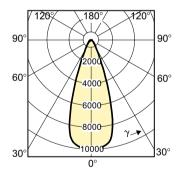
Light Distribution Diagram - MASTERC CDM-R 70W/830 E27 PAR30L 40D 1CT
