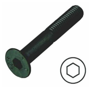
Countersunk socket screws are designed for light duty applications where there is limited space. These screws are widely used in many applications where a strong and reliable joint is required. Typically, countersunk socket screws are used to fasten plates and strips of metal to equipment and machinery as their flat head allows a flush, flat finish. This range of socket screws is made of mild steel and if painted or suitably treated these screws can be used outside.
