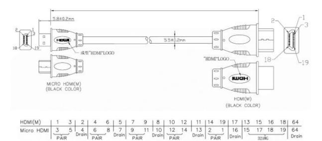
1. CABLE: 32AWG,UL20276,AL+B-FOIL,[(#32\*1P+D+FAM)\*5PCS+#32\*4C]+AM+B, BLACK COLOR,OD=5.5mm,PVC JACKET(Conductor: BC)(D: 30# CCS).
