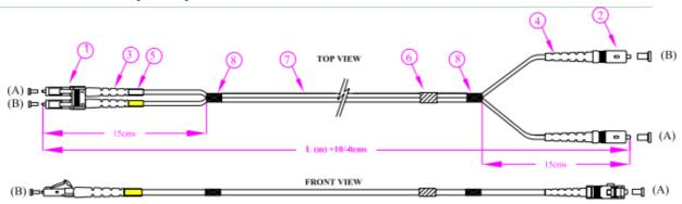
Connector: SC Clips shall be mounted to the connector to make it duplex.
