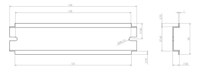
All dimensions are given within +/-0,5mm tolerance
