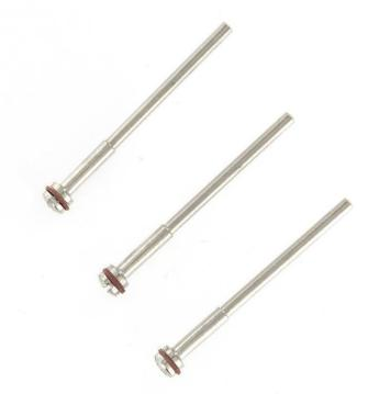
RS Pro mandrels usable with cuttings discs, mini circular saws, grinding wheels and rubberised abrasives. Simply unscrew the screw top, add the cutting wheel and tighten. Then fit the other end of the shank to the tool using the appropriate collet size.
