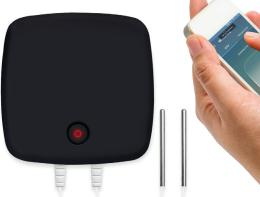
The PRO-MOTE-DTP+ kit has been designed to monitor temperature in a large range of applications, using High Accuracy 75mm length barrel temperature probes on 3m cables. Ideal for monitoring locations perhaps difficult or inhospitable to the data logger itself, the PRO-MOTE-DTP+ is ideal for monitoring refrigeration or storage units. This kit has 2 channels so you can monitor 2 separate areas simultaneously.
