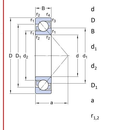
40 mm 80 mm 18 mm ≈ 56.25 mm ≈ 48.08 mm ≈ 65.55 mm 34 mm min. 1.1 mm
