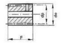
All dimensions in mm Standard tolerances, unless otherwise stated + - 0.25mm All worms are supplied with black oxide finish They are supplied with a M4 G/S fitted (5mm from one end) 1R=Single Start 2R=Double Start
