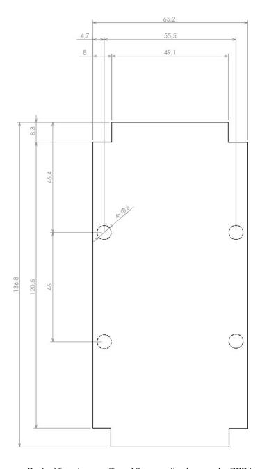
Dashed line shows outline of the mounting boss under PCB board Recommended mounting holes diameter ø3,5mm All dimensions are given within +/-0,5mm tolerance
