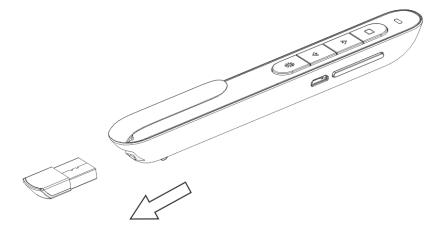
2)Plug the USB receiver into USB port.
