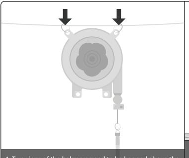
1. Two rings of the balancer need to be hanged above the working place to avoid dropping or tilting.
