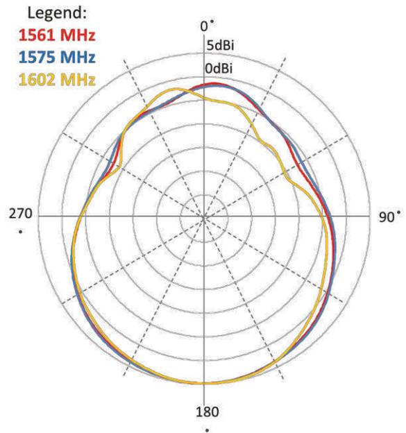
Data measured in free space and on reference ground plane of 70x70x1.0 mm ground plane condition, application data might vary.
