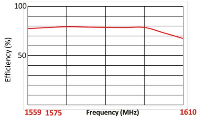
Data measured in free space and on reference ground plane of 70x70x1.0 mm ground plane condition, application data might vary.
