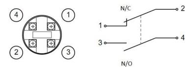
The switch is not polarity sensitive
