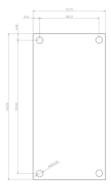
Dashed line shows outline of the mounting boss under PCB board Recommended mounting holes diameter ø3,5mm All dimensions are given within +/-0,5mm tolerance
