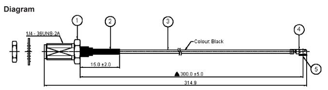
ItemDescription1RP-SMA B/H Jack for \$1.37mm Cable (Nut × 1, Washer × 1)2Heat Shrink Tube F32 \$2.5mm L = 15mm Colour: Black3\$1.37mm Cable Colour: Black4U.FL-LP-088 Shell for \$1.37mm Cable5U.FL-LP-088 Terminal for \$1.37mm Cable
