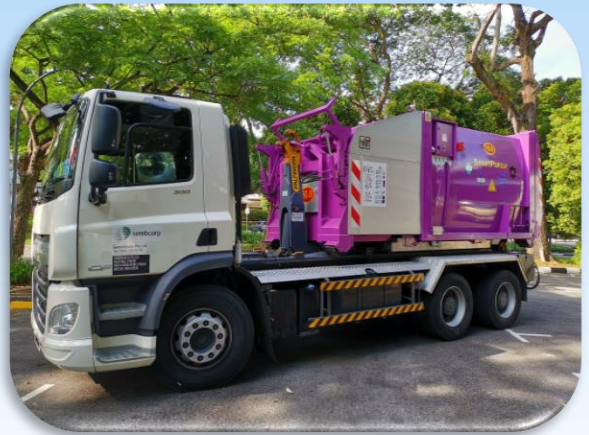
Hooklift truck deploys to site upon receiving 85% full alert
