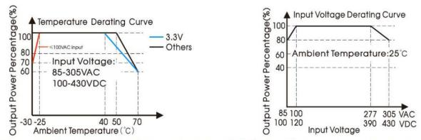
Note: 1. With an AC input between 85-100V/277-305VAC and a DC input between 100-120VDC/390-430VDC, the output power must be derated as per temperature derating curves;
