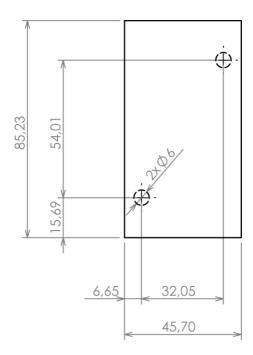
Dashed line shows outline of the mounting boss under PCB board Recommended mounting holes diameter ø3,5mm
