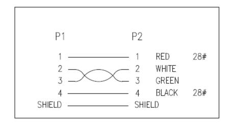
USB 2.0 CABLE, UL STYLE 1 TWISTED PAIR 28AWG AND 2C 28AWG,OD 3.5mm, AMA BRAID, JACKET BLACK, DRAWING No. EUAB2801P2802C-146
