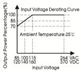
Note: With an AC input voltage between 85-115VAC and a DC input between 120-160VDC the output power must be derated as per the temperature derating curves.
