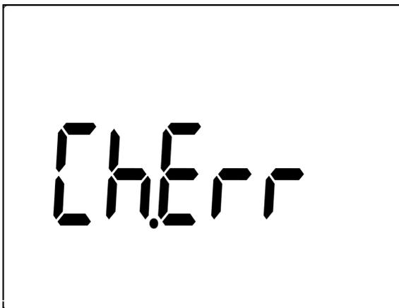
**Figure 6-3** Charge terminal alert
