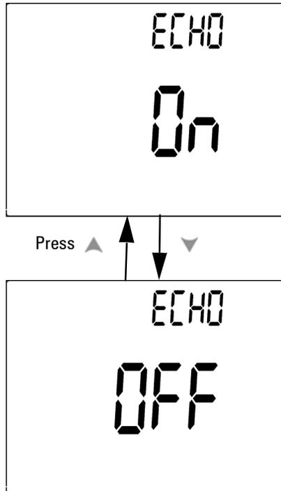
**Figure 4-14** Echo mode setup for remote control
