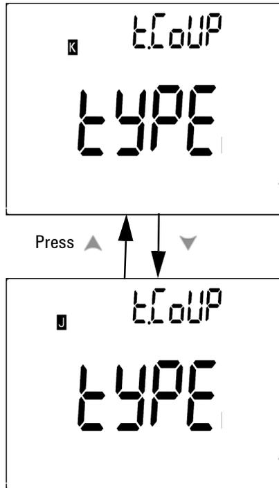
**Figure 4-3** Thermocouple type setup
