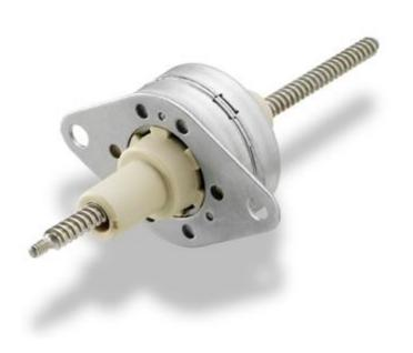
A non-captive linear actuator that provides a long stroke length and up to 128 oz of linear force in a 26 mm frame size. The 7.5 degree step angle and option of 0.0005" lead screw pitch options allows for greater positional resolution.
