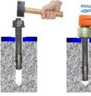
Insert assembled anchor through fixture into concrete
