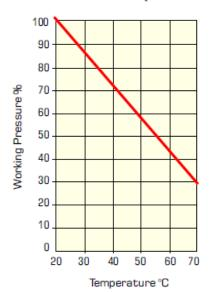
Max. recommended continuous working temperature = 60°C
