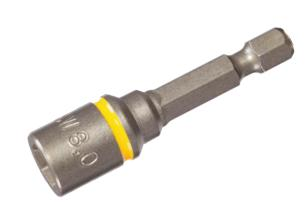
RS Pro Magnetic Impact Nut Setter for driving hex head screws when using an impact driver with an impact effect. The magnetic insert in the nut setter holds the fastener into the tool which frees up the users hands, especially useful in tight and awkward applications. The tool is colour coded for easier size identification. Supplied in a compact plastic box.
