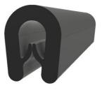
**Description:** Black Nitrile Rubber with steel wire insert. Provides edge protection to sheet material and reduces noise and wear resulting from vibrations. Oil Resistant Temperature range -40 to +100°C.
