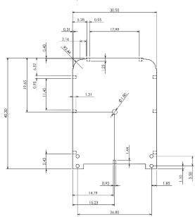
All dimensions are given within +/-0,5mm tolerance
