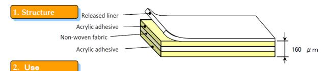
1) To adhere to resin plate and punching process.
