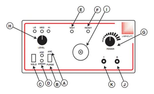
A Arc B Purge Argon gas and weld current controlled by the "Weld" switch. LED indication Allows the gas line and electrode shield to be purged of air prior to a new welding period
