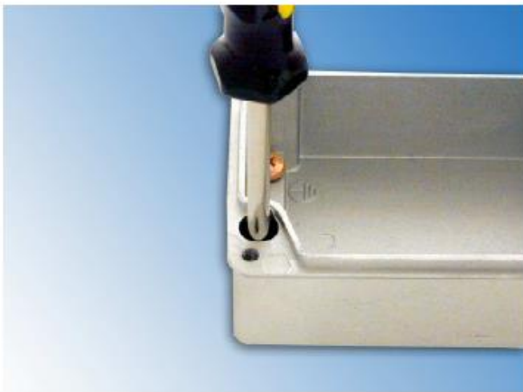
The enclosure can be fixed by means of normal screws inserted in through holes with screw head bearing on the bottom and outside the gasketed perimeter. The protection degree of the gasketed remains unchanged.
