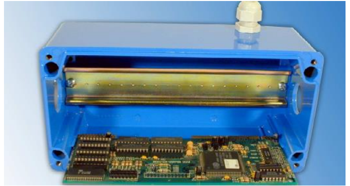
Inside the enclosures of GAIN type there are supports provided with holes for screwing the OMEGA DIN 46277 sections, supplied by request (see accessories of EGO series). One or more slides, depending on the dimensions of the enclosure, allow the insertion of printed circuit boards (as illustrated at pages 12 and 13)
