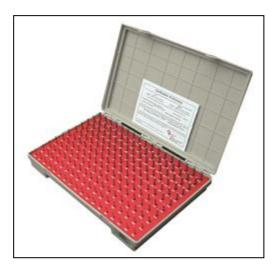
High precision pin gauge set are suitable for a range of uses: Checking hole size, slot widths, distance between holes, Go and No Go size, setting micrometers and other gauges Fully hardened: HRC 60-62 Pin length: 2" Surface finish: 10 micro inches or better Roundness: within 0.0001" Sizes and tolerance direction marked on gauges above 0.060" and 1.28mm All sets contain a certificate of accuracy
