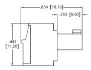
Positions: 02 thru 24 A = .150 [3.81] x No. of Spaces + .181 [4.60] B = .150 [3.81] x No. of Spaces
