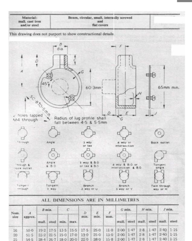
NOTE. Dimension G applies to unmachined parts only.
