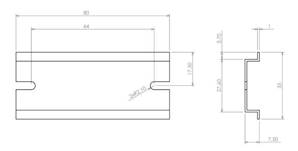
All dimensions are given within +/-0,5mm tolerance
