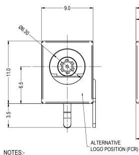
1. SUITABLE FOR USE WITH Ø2.1mm OR Ø2.5mm DC PLUG.
