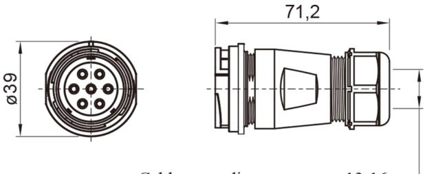
Cable outer diameter range: 13-16mm
