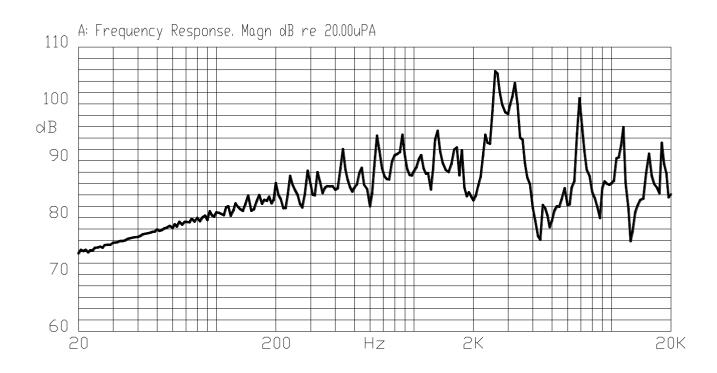
S.P.L. Measuring Circuit Input Signal: 10Vp-p,800Hz, Square Wave
