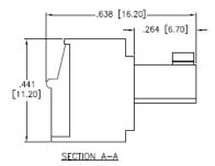
Positions: 2 thru 24 A = .138 [3.50] x No. of Spaces + .169 [4.30] B = .138 [3.50] x No. of Spaces
