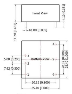
Note: Unit: mm[inch] Pin diameter tolerances: ±0.10[±0.004] General tolerances: ±0.50[±0.020]
